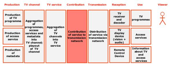
A television contribution network is a closed digital network that delivers the signal from the broadcaster's play-out system to the distribution network delivering digital television to the viewers.
